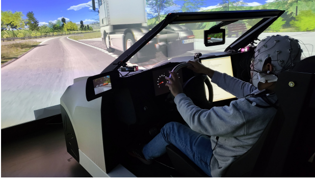
Fig. 2: Illustration of participant with EEG set up in the driving simulator.
