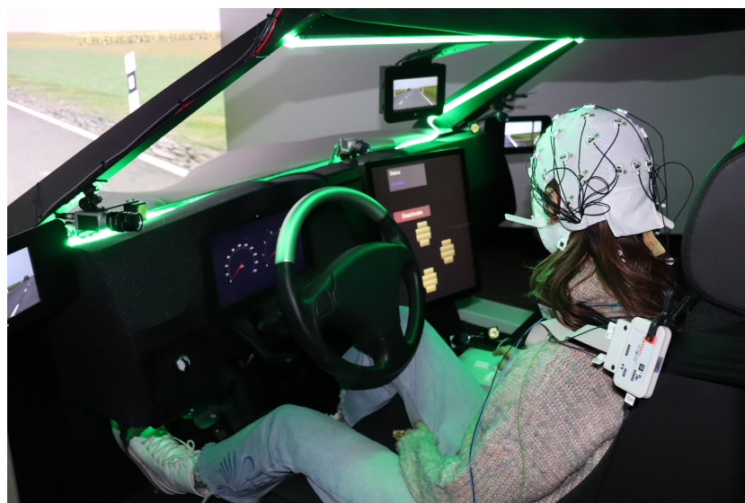
Figure 1. The vehicle mock-up with LED light around the windshield and NDRT presented on the dashboard screen
